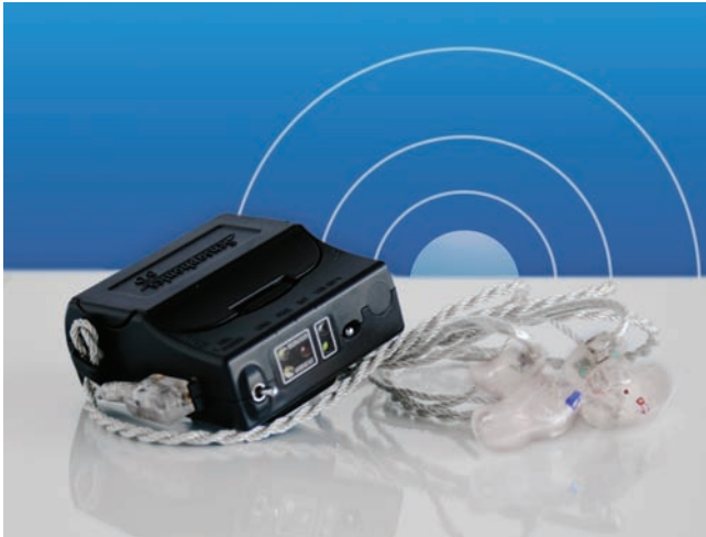
The state of the art in IEMs is the 3D Active Ambient, offering full isolation while capturing ambient sound with microphones embedded in the earpieces.
